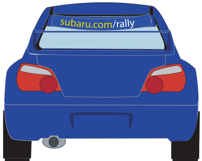
subaru.com/rally banner logo Place along top of rear windshield Decal is cut to fit curvature
